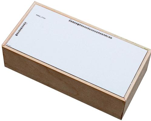
Figure 5. Capacitive sensing surface with piezoelectric microphone
