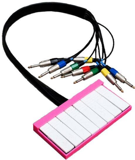
Figure 1. 3D printed keys with individual microphones
